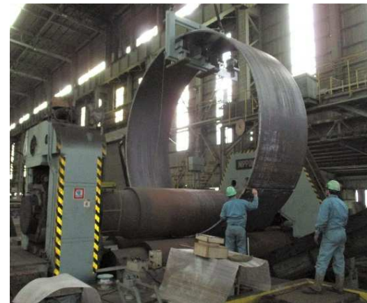
Bending Operation by Large Bending Roll
