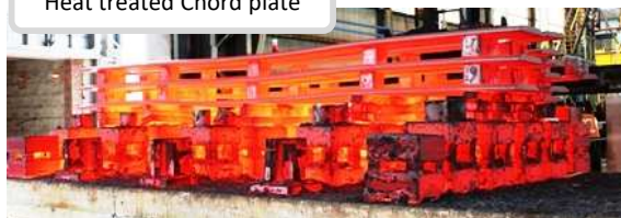
Heat treated Chord plate
