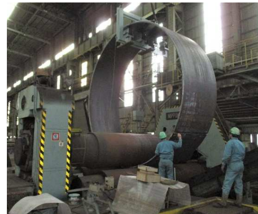
Bending Operation by Large Bending Roll
