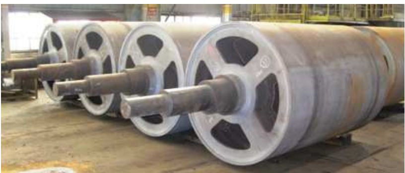
Hearth Roll for Continuous Annealing Equipment (CAPL)
